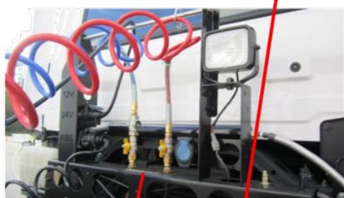
Sample of optional features shown from a Dealership with the primemover's air supply lines, taps and electrical leads set up with a catwalk tread plate.
