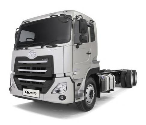
GH11TB - 294 kW (400 PS) @ 1600 rpm Power:
